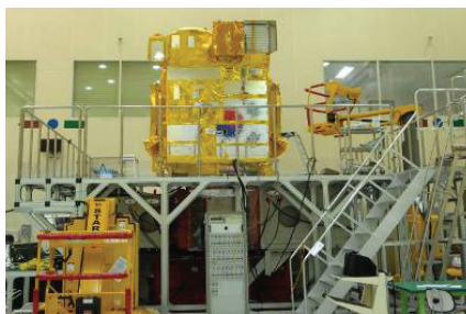
(c) Triple vertical shaker system
