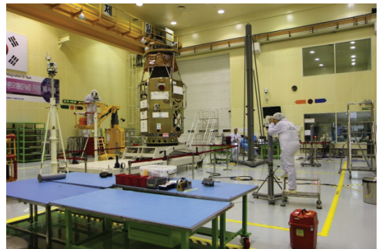
[그림 5] System alignment measurement of satellite
